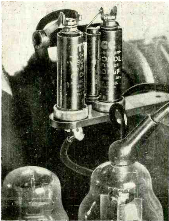
Close-up of booster unit mounted close to the line-scan output valve.
